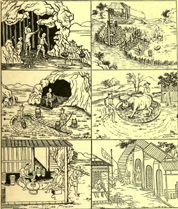
1. Quarrying. 2. The pounding mill. 3. Further pounding in a trough. 4. Kneading by buffaloes. 5. The potter's wheel. 6. The kilns.
